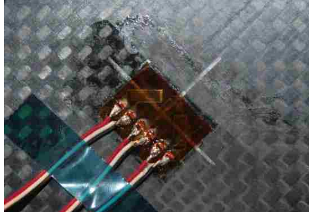
Figure 3.15: Strain gage rosette placement on PFS sample.
