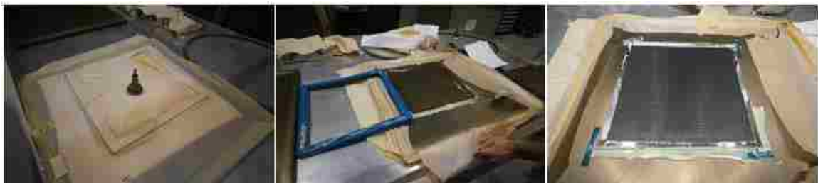
Figure 3.12: Debaggging of cured composite plate.
